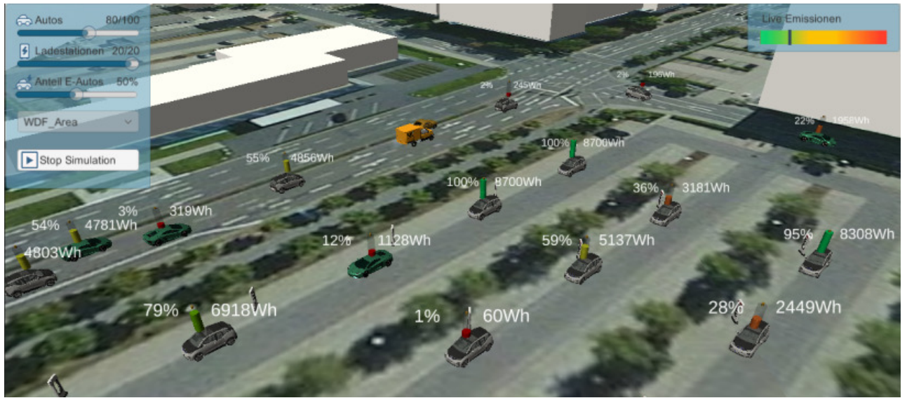
Fig. 3. Visualization in Unity 3D of incoming EVs and their allocation to the parking charging stations
