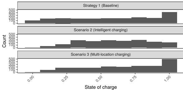
Figure 6. Distribution of SoC in each strategy simulated with 2000 EVs
