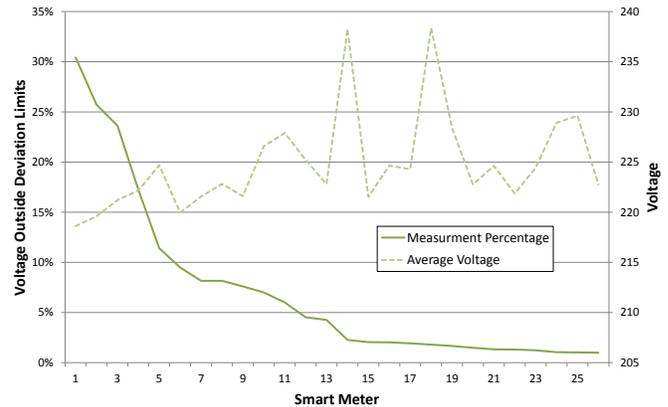
Figure 5. Measurements with voltages outside lower deviation limit
