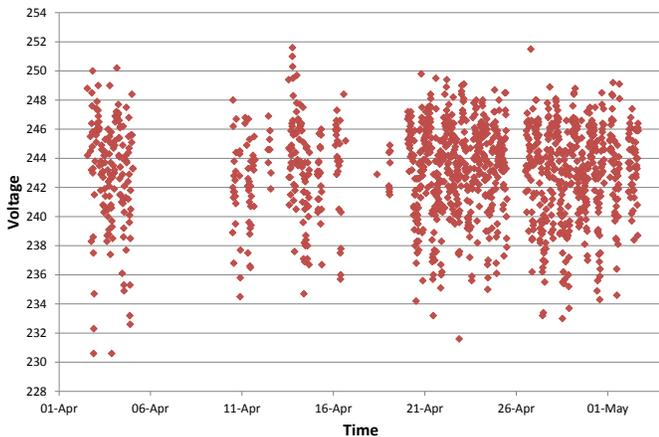
Figure 4. Example of a device violating the higher voltage boundary
