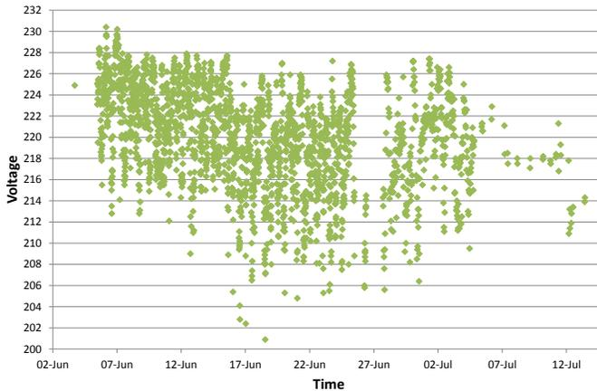
Figure 3. Example of a device violating the lower voltage boundary
