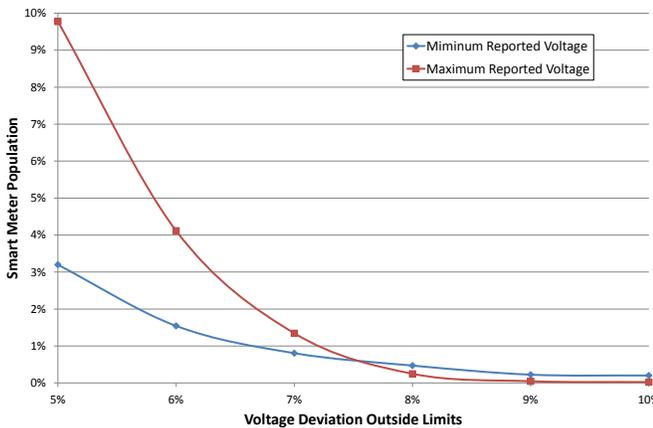
Figure 7. Device distribution near to and exceeding deviation limits
