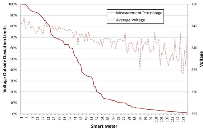
Figure 6. Measurements with voltages outside higher deviation limit
