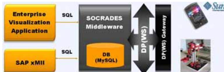
Figure 2 – Integration of Enterprise, Middleware and Device layers
