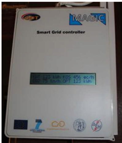
Figure 4: The intelligent load controller used by the MAGIC system in field test C.
